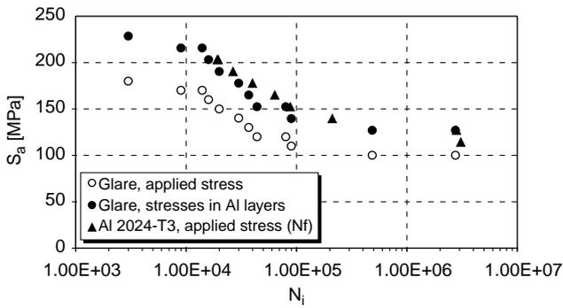
Fig. 7. Comparison of fatigue initiation lives between Glare 3-3/2-0.3 and 2024-T3 un-notched specimens at RT. Stresses in Glare are related to the overall applied stresses as well as to the stresses in the aluminium layers.
