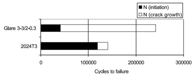
Fig. 4. Contributions of different phases to the total fatigue life in Glare 3-3/2-0.3 and 2024T3 for an open hole specimen and fatigue load as shown in Fig. 2.
