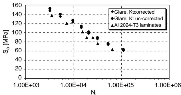
Fig. 10. Comparison of fatigue initiation lives between Glare 3-3/2-0.3 and 2024-T3 notched specimens at RT. Stresses in Glare are related to the aluminium layers, with and without the correction for anisotropy effects in the stress concentration factor.
