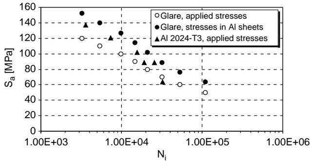
Fig. 9. Comparison of fatigue initiation lives between Glare 3-3/2-0.3 and 2024-T3 notched specimens at RT. Stresses in Glare are related to the overall applied stresses as well as to the stresses in the aluminium layers.
