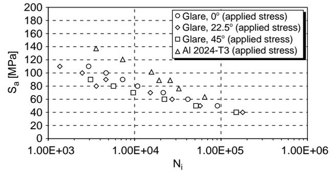
Fig. 11. Comparison of fatigue initiation lives between Glare 4B-3/2-0.3 under different off-axis angles and 2024-T3 laminates at RT. Stresses in Glare are related to the overall applied stresses.
