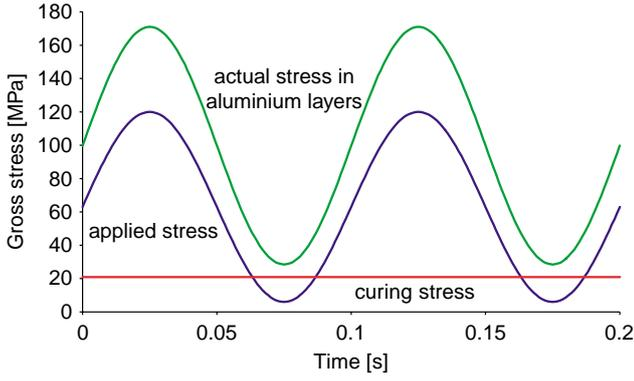
Fig. 5. The stress cycle in the aluminium layers of a Glare 3-3/2-0.3 laminate loaded in  $L$  direction at RT is a superposition of the stress cycle induced by the applied stress and the curing stress [6].
