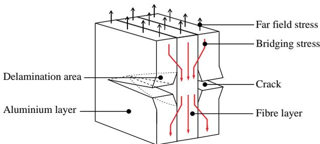
Fig. 1. Crack bridging of the fibres and delamination of the layers.
