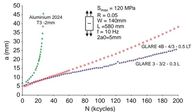
Fig. 2. Crack growth curves of aluminium 2024-T3, Glare 3-3/2-0.3 L and Glare 4B-4/3-0.5 LT for constant amplitude fatigue loading [3].
