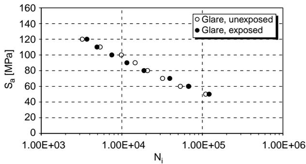
Fig. 13. Comparison of fatigue initiation lives between Glare 3-3/2-0.3 exposed (3000 h, 70 °C, 85% humidity) and unexposed. Stresses in Glare are related to the overall applied stresses.
