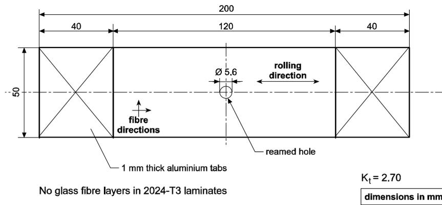
Glare 3-3/2-0.3 and 2024-T3 laminate specimens used in fatigue crack initiation tests on notched specimens
