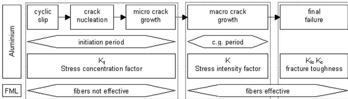
Fig. 3. Different phases of the fatigue life in Fibre Metal Laminates together with relevant factors.
