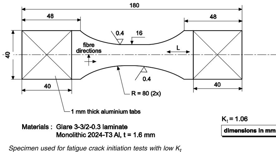
Fig. 6. Un-notched fatigue specimen.
