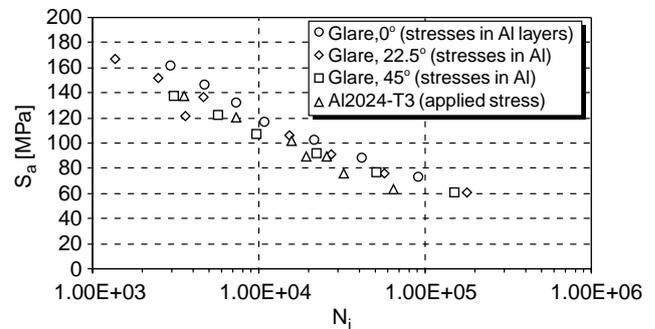
Fig. 12. Comparison of fatigue initiation lives between Glare 4B-3/2-0.3 under different off-axis angles and 2024-T3 laminates at RT. Stresses in Glare are related to the aluminium layers.
